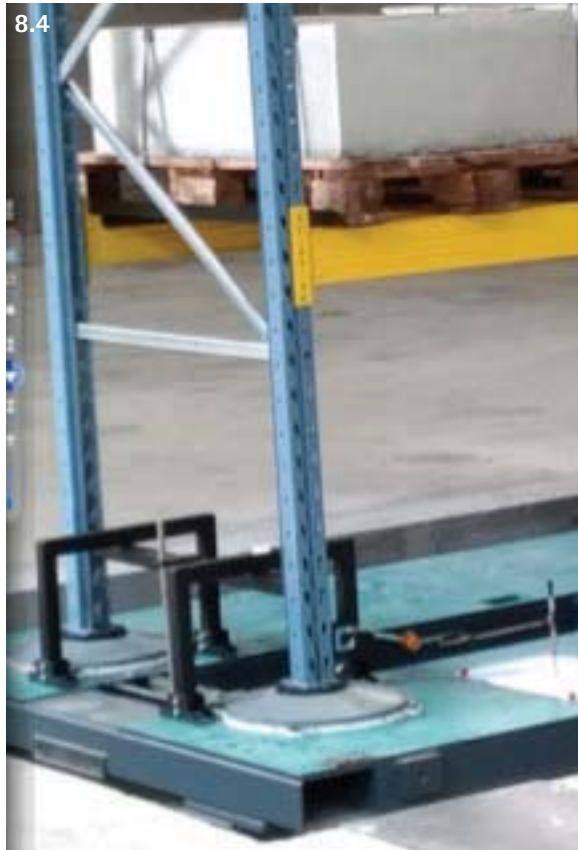
Picture 8.1 – Cyclic flexural testing on LOKI devices by ALGA. Picture 8.2 – Shaking table testing on LOKI devices by National Technical University of Atene Picture 8.3 – Shaking table testing on LOKIBASE devices by Girardini Laboratory. Picture 8.4 - Shaking table testing on Pallet Racking System (with LOKIBASE devices) by Girardini Laboratory. Picture 8.5 – Cylindrical beam damper with double-circular cross section.
