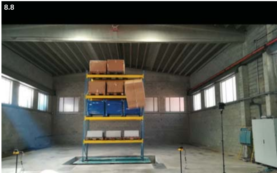
Picture 8.6 - Shaking table testing on Wine Barrel Rack (with LOKIBASE devices) by Girardini Laboratory. Picture 8.7 - Shaking table testing on Wine Barrel Rack (without LOKIBASE devices) by Girardini Laboratory. Picture 8.8 -Shaking table testing on Pallet Racking System (without LOKIBASE devices)by Girardini Laboratory. Picture 8.9 -LOKI device. Picture 8.10 - Cylindrical beam damper with double- circular cross section.
